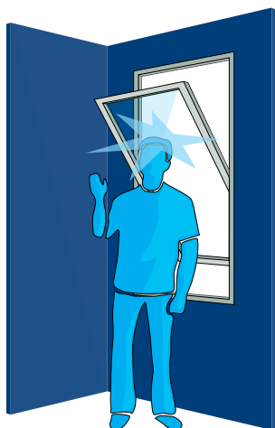
Risk of injury caused by sash impact.
